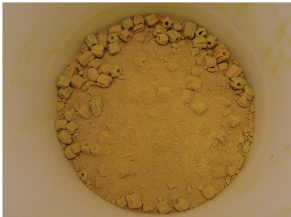
Fig. 2: A sample of degraded catalyst comprised mostly of dust.
