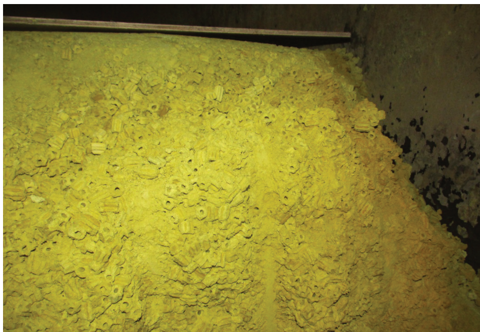
Fig. 1: Solidified catalyst bed due to structural degradation.
